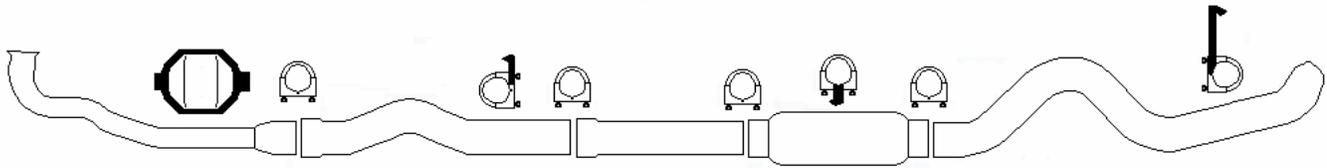
Note: this kit was designed for non-catalyst equipped 92-93 models. These models had metal strap hangers. On 94+ vehicles, rod hangers were used. For those with the 94+ models with rod hangers, alternate hanger setups will need to be made for use of this kit on the vehicle, the rod hangers are not included in this kit.
